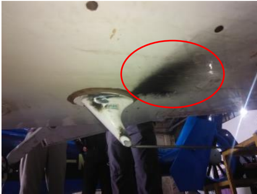
Fig:31 - Burn marks on belly
